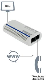
d. If the telephone set is connected to the 56Kbps USB modem via a telephone cord, lift the telephone handset, and check for a dial tone.
